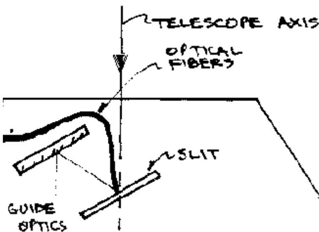
It all starts with the telescope light beam entering the spectrometer. The focal point of the telescope beam is brought to the *slit* of the spectrometer. **This slit is what is ultimately imaged on the detector.** In the case of the Camp spectrometer, the slit is arranged at an angle and the slit surroundings are silvered so that the portion of the telescope beam not passing through the slit can be routed instead to an eyepiece for
