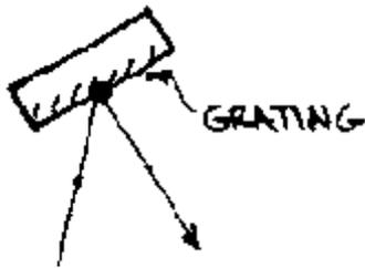
... to the *diffraction grating*! This optical element disperses the parallel beams of light into their component colors/wavelengths/energies. Each different wavelength comes off of the grating at a slightly different angle. So now, we have an image of the slit that is spread out like a rainbow by color.
