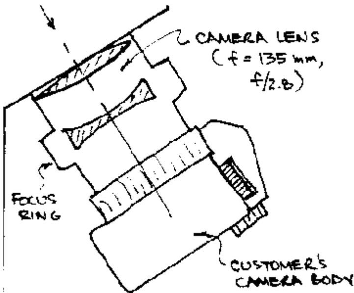
This new color-dispersed beam of light is then focused and imaged on the detector by the *camera lens*. A 35 mm camera is the detector in this diagram, but at Camp, we typically use an eyepiece or a CCD array.
