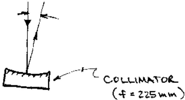
The light passing through the slit then is reflected off a *collimating mirror*, which parallelizes the beam of light, before sending it off...
