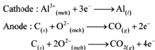
If a metal is used instead of graphite as the anode, then  $\text{O}_2$  will be liberated. This will not only oxidise the metal of the electrode, but also convert some of the Al liberated at the cathode back into  $\text{Al}_2\text{O}_3$ . Hence, graphite is used for preventing the formation of  $\text{O}_2$  at the anode. Moreover, graphite is cheaper than other metals.
