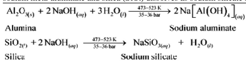
The impurities are then filtered and the solution is neutralized by passing CO<sub>2</sub> gas. In this process, hydrated Al<sub>2</sub>O<sub>3</sub> gets precipitated and sodium silicate remains in the solution. Precipitation is induced by seeding the solution with freshly prepared samples of hydrated Al<sub>2</sub>O<sub>3</sub>.
