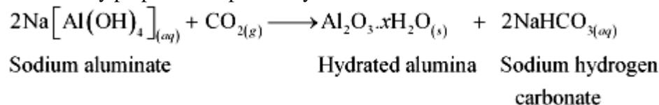
During this process, sodium silicate remains in the solution. The obtained hydrated alumina is filtered, dried, and heated to get back pure alumina.
