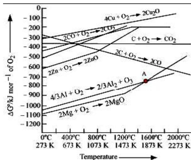
The above figure is a plot of Gibbs energy ( $\Delta G^\ominus$ ) vs. T for formation of some oxides. It can be observed from the above graph that a metal can reduce the oxide of other metals, if the standard free energy of formation ( $\Delta_f G^\ominus$ ) of the oxide of the former is more negative than the latter.
